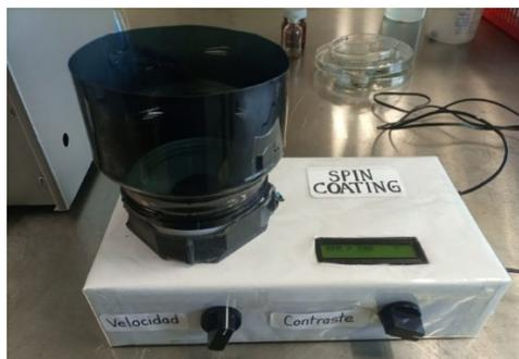
Figura 3.1 Prototipo final de spin coating.
