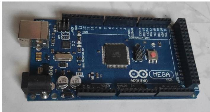
Figura 24: Arduino Mega
