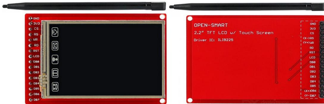
Figura 3.3 OPEN-SMART 2.2" TFT LCD
