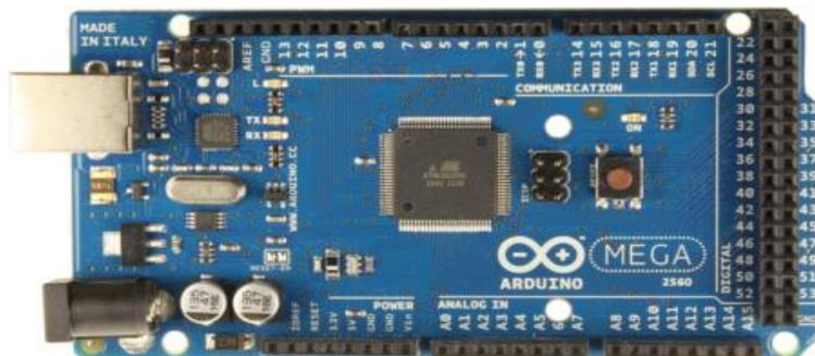
Figura 2.2 Arduino Mega 2560
