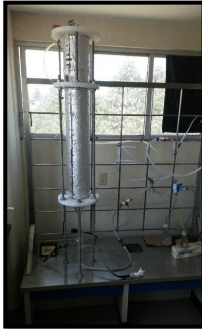
Figura 2.11. Reactor O 3 /UV
