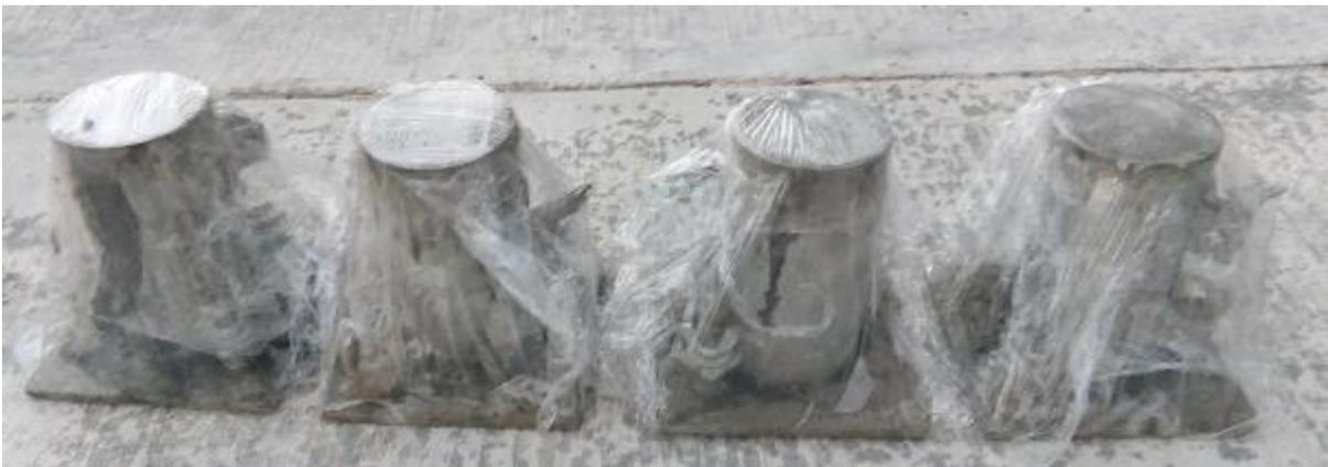
Figura 3.38 Cilindros de concreto experimental 15 cms.
