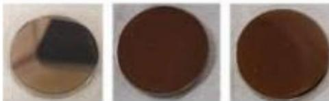
**Figure 3** 316L stainless steel substrates after Ti/TiN deposition by PVD
