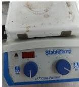
A magnetic stirrer with a digital display and two control knobs. The brand name 'StableTemp' is visible on the front panel. |
