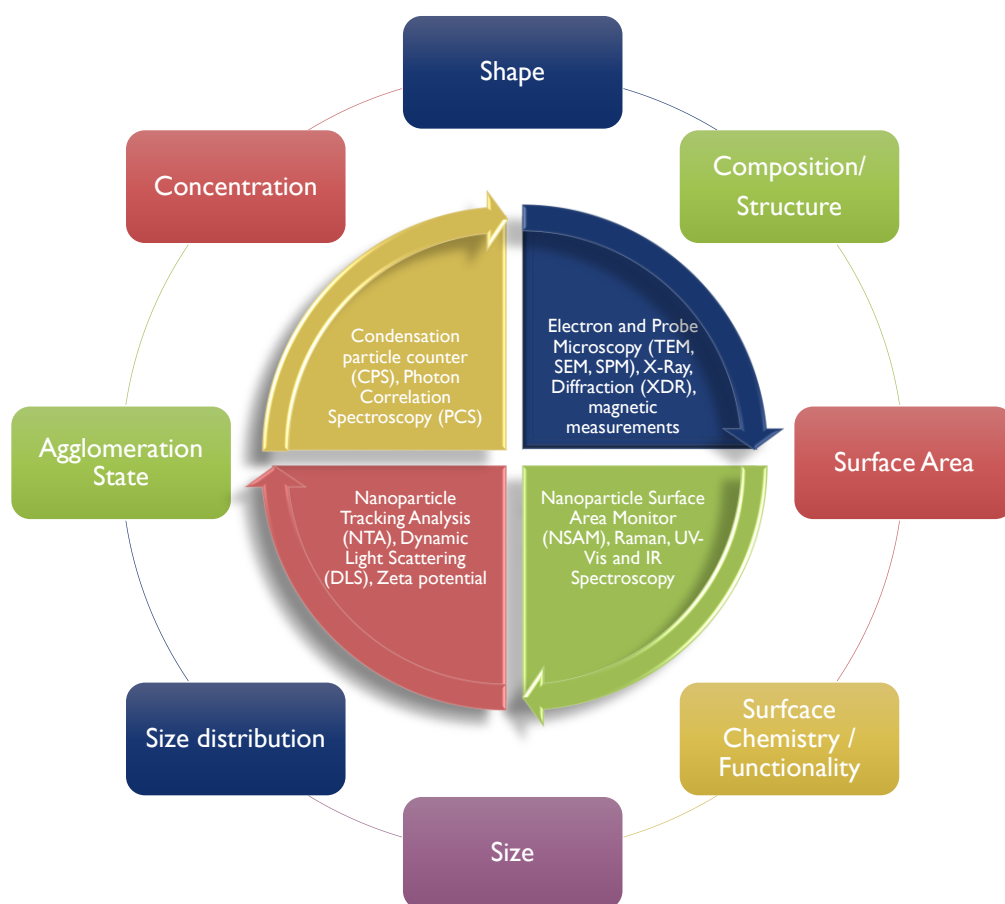
Figure 2.1 Scheme of typical characterization techniques used with nanoparticles. 1,2
