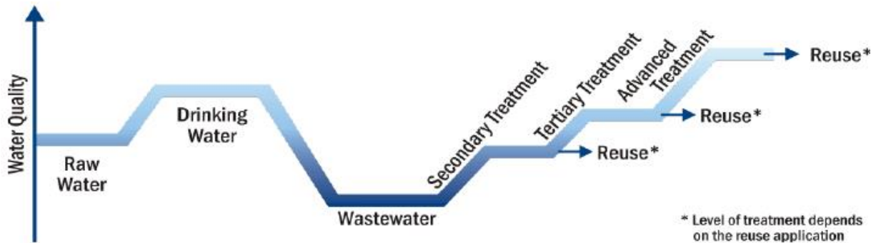
Figure 3.1 Treatment technologies to achieve any desired level of water quality. 8
