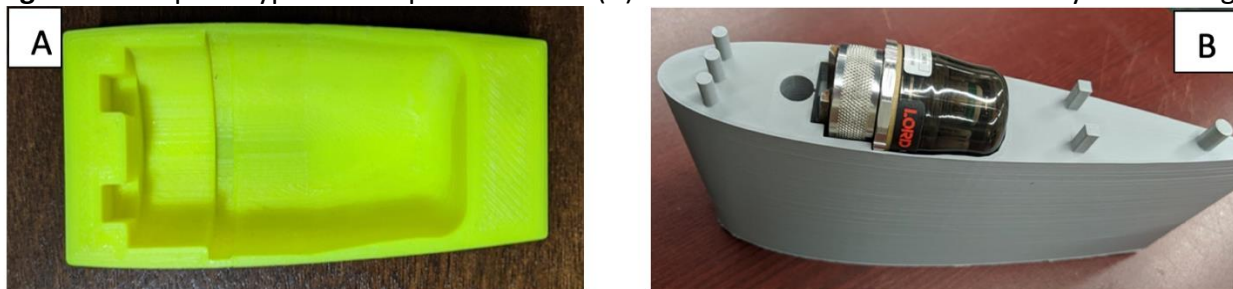
Figure 5. The prototype of the spot for sensor (A) and the vibration sensor assembly in the wing
