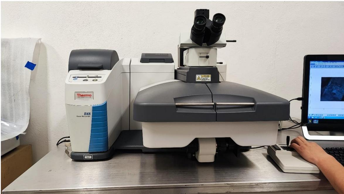
*Figura 15 Microscopio Raman Confocal Thermo Scientific™ DXR™ 2*
